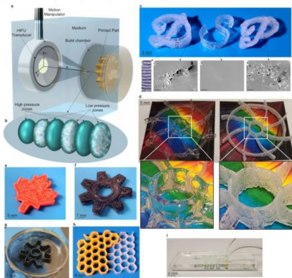
Fig. 1: DSP concept and printed parts.
